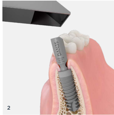
2 Place the scan body with hand-torque (max. 5 Ncm) into the implant and scan intraorally. Send scan data to the dental laboratory.
