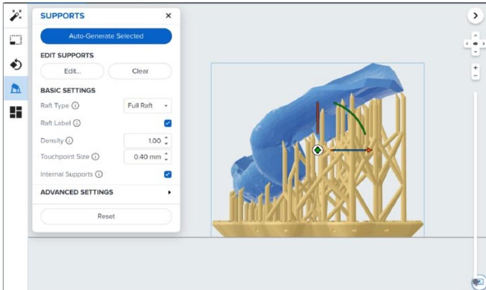
To allow for simple and precise assembly, ensure that there are no supports (white dots) on the patient-contacting surfaces. Use the manual support editing feature to closely inspect support locations and add or remove supports as needed.
