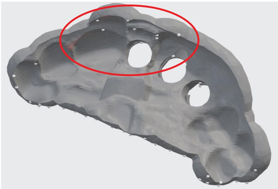
To allow for simple and precise assembly, ensure that there are no supports on the inner side or in the inside of the guide sleeve opening. Use the manual support editing feature to closely inspect support locations and add or remove supports as needed.
