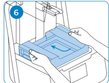
A sensor detects the resin tank, and the status light illuminates. **6**
