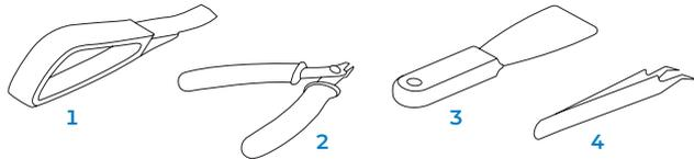
The accessories include sharp tools such as: a part removal tool (1), flush cutters (2), a scraper (3), and tweezers (4).
