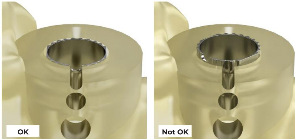
Use magnifying aids like microscope or camera to make sure that the guide sleeve is in the correct position. Visually inspect that the coronal surface of the guide sleeve is flush and level with the surface of the guide sleeve opening, which confirms correct depth and angulation of the guide sleeve.
