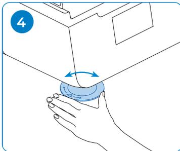
5. Adjust the feet until the touchscreen indicates the printer is level.
