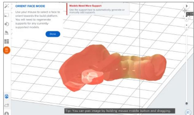
Subsequently, the face surrounding the sleeve should be oriented under an angle of + or - 30° with the build plate to optimize accuracy. The distal ends of the guide should be pointing away from the build plate, wherever applicable.
